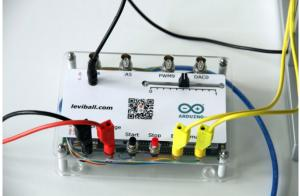
An IR-sensor measures the gap between coil and ball and software routines calculate and control, using these gap signals, the power supply of an electromagnet to levitate the ball.
